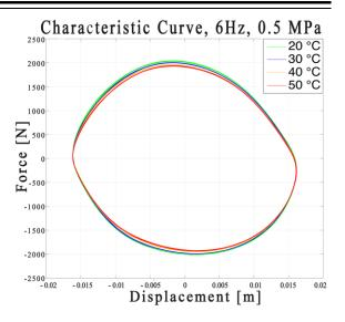
Fig. 12. Characteristic Curve, 6Hz, 0.5MPa, [20-30-40-50 °C]
