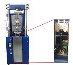
Fig. 2. The test bench and a detail of its road crank
