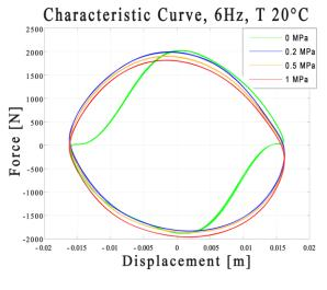
Fig. 5. Characteristic Curve, 6Hz, [0 - 0.2 - 0.5 - 1 MPa]
