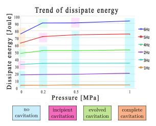
Fig. 14. Variation the performance of the shock absorber
