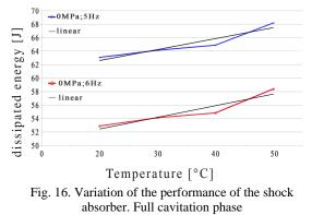
From Figure 16, it arises that the increase trend is the same: the curve is only translated by the different stress level. For a variation of 40°C, the shock absorber retrieves an 8% of its performance.
