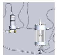
Fig. 3. Render of the transparent monotube shock absorber
